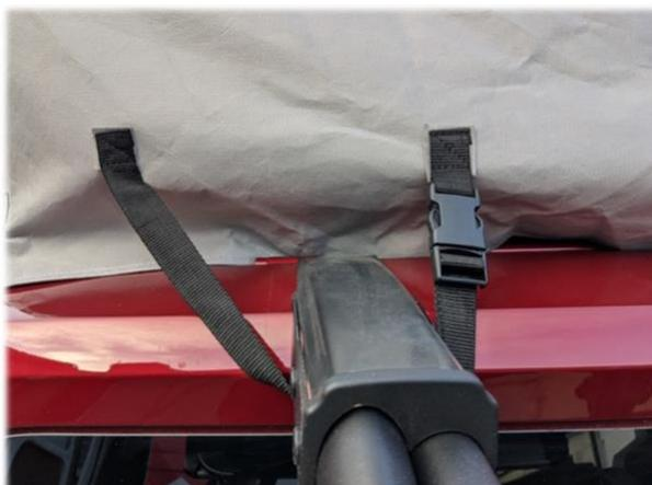
Your Vanorak will fit securely to your Volkswagen California providing increased insulation and protection to the roof bellows. To remove the cover simply follow the instructions in reverse, remembering to undo all clips prior to lowering roof, then remove the rear corners first for ease of removal.
